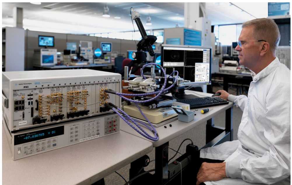
Figure 1: Adding two-port PXI VNA modules to an existing test station enables powerful device characterization without expanding system height or footprint.
