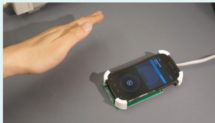
The SideSwipe system uses the phone's transmissions to sense nearby gestures. Credit: University of Washington.
